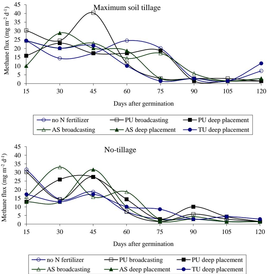
**Figure 1.** Pattern of methane flux from soil tillage system and N fertilizer management in rice fields in Pati district, Indonesia, for the 2019 dry season. PU: Prilled urea; AS: ammonium sulfate; TU: tablet urea.
