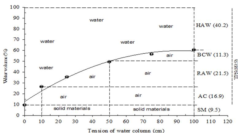
**Figure 1.** Water release curve of the substrate (peat moss and tezontle in a 3:1 v:v ratio) from 0 to 10 kPa (based on De Boodt et al., 1974). HAW: Hardly available water; BCW: buffering capacity water; RAW: readily available water; AC: air capacity; SM: solid materials; TPS: total pore space.
