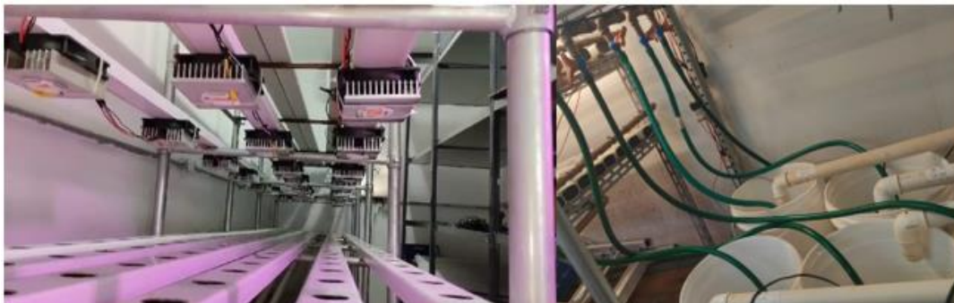
Figure 2. Details of the hydroponic bench with lights and hydroponic profiles and individual solution reservoirs.
