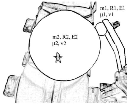
$m_1$  = mass of impacting sphere;  $m_2$  = fruit mass;  $\mu_1$  = Poisson's ratio of impact sphere;  $\mu_2$  = Poisson's ratio of fruit;  $E_1$  = modulus of elasticity of impacting sphere;  $E_2$  = modulus of fruit elasticity;  $R_1$  = radius of curvature at contact point of impacting sphere;  $R_2$  = radius of curvature at contact point of fruit.
