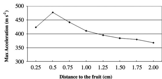
**Figure 5. Deceleration variation according to impact distance.**
