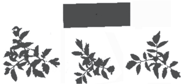
Figure 2. Example of the processed image from the image analyzer along with the standard 150 cm 2 area.
