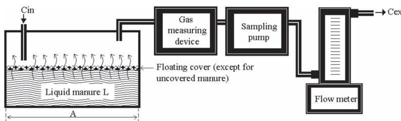
Cin: Gas concentration of air inlet into the chamber; Cex: gas concentration of air outlet from the chamber.
