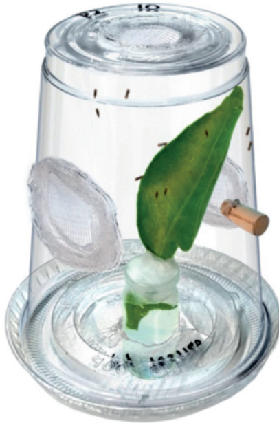
Figure 1. Bioassay arena used in the laboratory to evaluate the potential repellent effects of plant oil extracts on Diaphorina citri adults.
